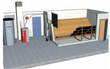
**Auger/Pneumatic**—ideal for rectangular rooms with front-end removal. Complete emptying guaranteed due to deep and horizontal position of the delivery screw. Use with the suction system for flexible boiler setup.
