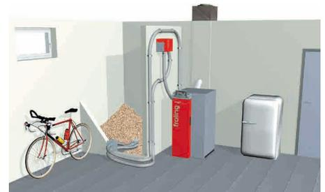
**Universal Suction**—one or three suction probes uniformly provides complete emptying of the pellet store room.
